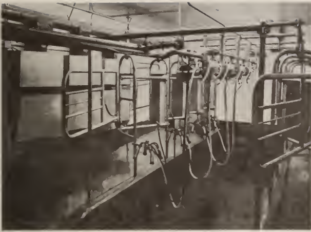
All the equipment — herringbone stalls — Universal Milking System — Feed-a-Meter — Milk-a-Meter — ready and waiting for the star performers to come on stage.
